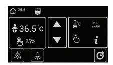
In MANUAL MODE, the warmer provides user-adjustable heater power and the option to monitor the baby's skin temperature using skin sensor.
