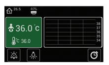
In BABY MODE, the warmer provides stable control of the baby's skin temperature by automatically adjusting the heater power to compensate for varying physiological and environmental conditions.
