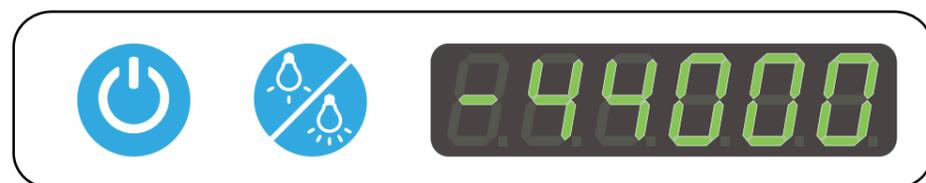
If the Colibri Phototherapy has been used for over 44 000 hours, after turning ON the display will show the “total device hours” for 3 seconds and ‘Error 4’ message after that. The error message will continue to appear every second during treatment.
