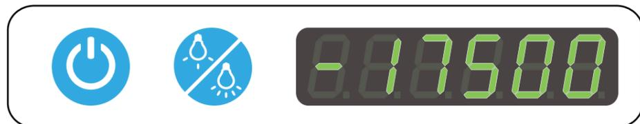
The display shows the "total device hours". This will be displayed for 3 seconds.
