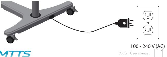
The connector plugs into the back of the Colibri Photothrapy base and then directly into the power outlet in
