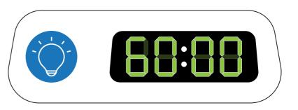
After turning ON the Firefly the display will show the "total device hours" This particular example shows 60,000 hours.
