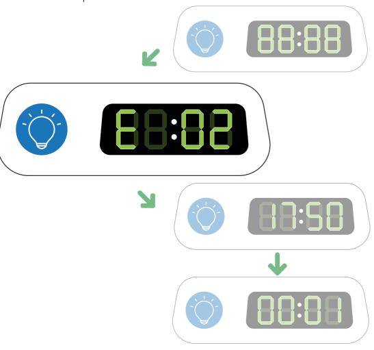
The image above shows when exactly in the 'start-up' process the error message will be displayed.
