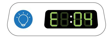
At 60,000 hours and anytime after 60,000 hours E04 code will be displayed. This indicates that the LED's have reached the recommended life span. This message will appear for 5 seconds after the device is switched on following total number of hours displayed for 3 seconds. After that E04 and total number of hours will alternate 1 second each.
