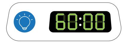
After turning ON the Firefly the display will show the "total device hours" This particular example shows 60,000 hours.
