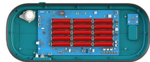
Access the batteries located at the bottom of the base.
